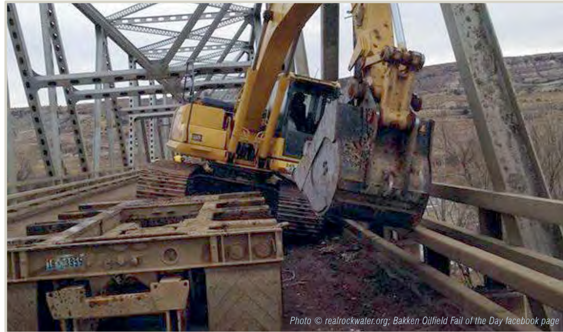
Figure 84, Load shifted off trailer after collision with Long X Bridge overhead member
