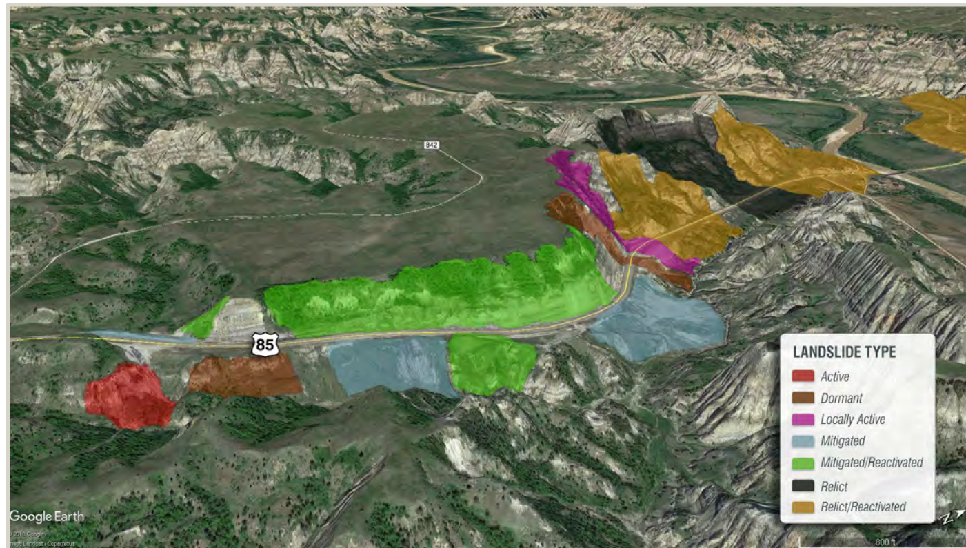
Figure 55, Google Earth Aerial Image of Mapped Landslides (Long X Bridge)
