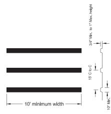
PORTABLE RUMBLE STRIPS ARRAY DETAIL
