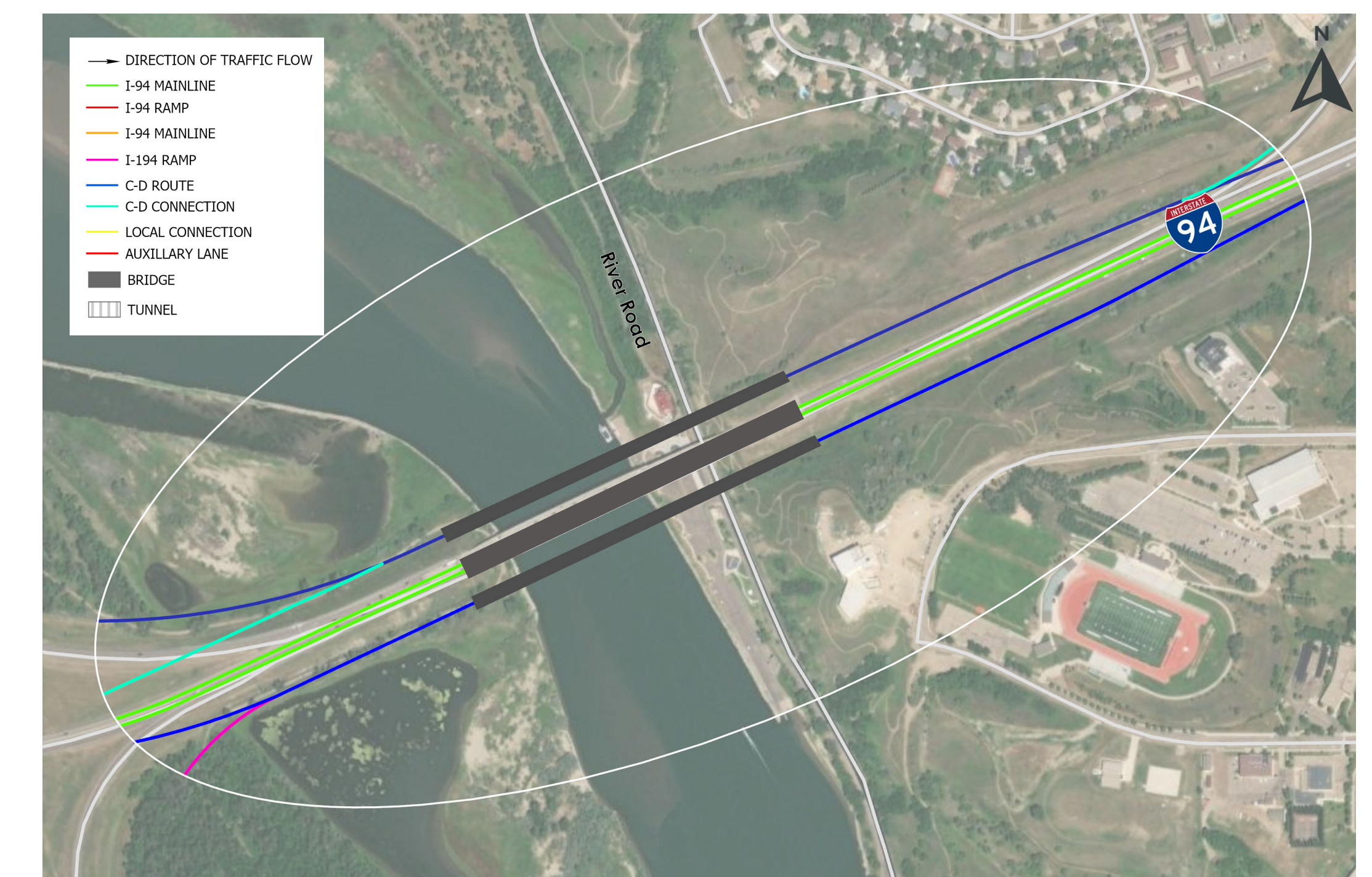
1. C-D freeway lanes and bridges over the river with I-94 westbound flyover added to reconstructed bridge.
