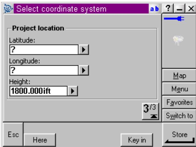
Project Height should be within 100ft of actual elevation.
