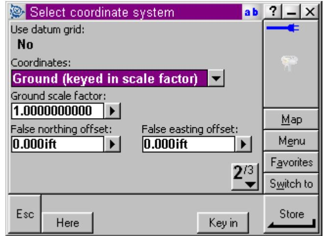
**All Survey Data will be collected using Grid Coordinates. For final Ground Coordinate data submission, data will be converted to ground per “Design to Construction Automation” Manual beginning on page 19**
