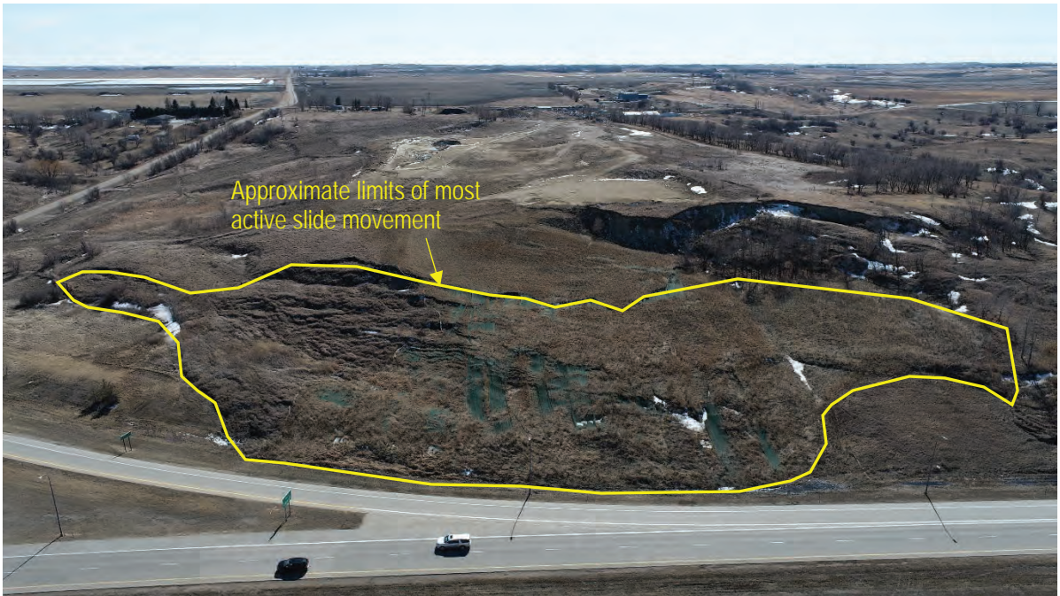
Exhibit 3-1: Site Reconnaissance Photo 1 - Overview of the landslide complex taken from the north side of Interstate 94, looking south. Green fabric on the slope is an erosion control blanket/turf reinforcement mat (TRM) placed during a grading project in 2019.
