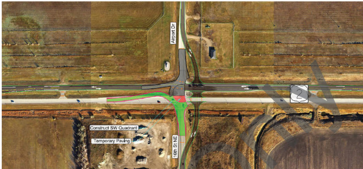
Figure 12: Work Zone Traffic Control Phase 3
