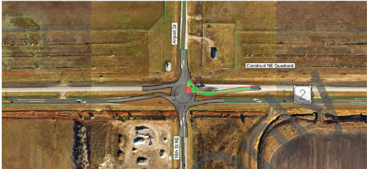
Figure 14: Work Zone Traffic Control Phase 5
