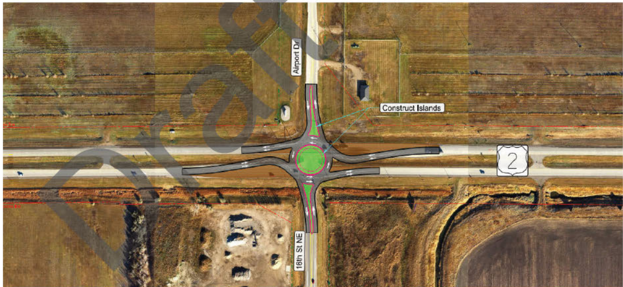
Figure 15: Work Zone Traffic Control Phase 6
