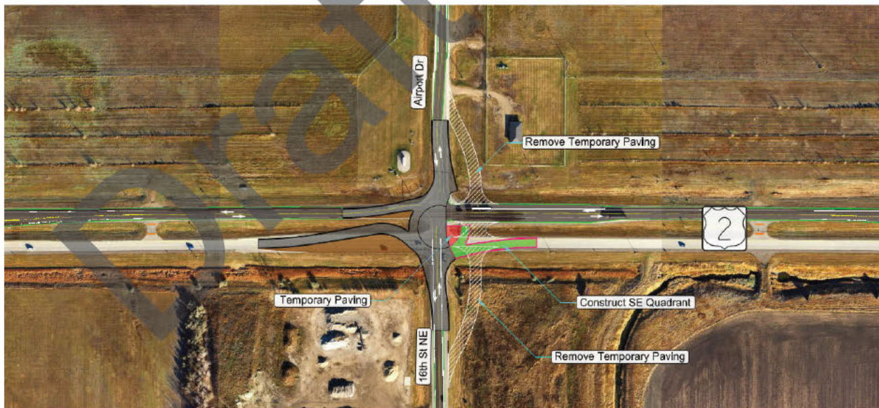
Figure 13: Work Zone Traffic Control Phase 4
