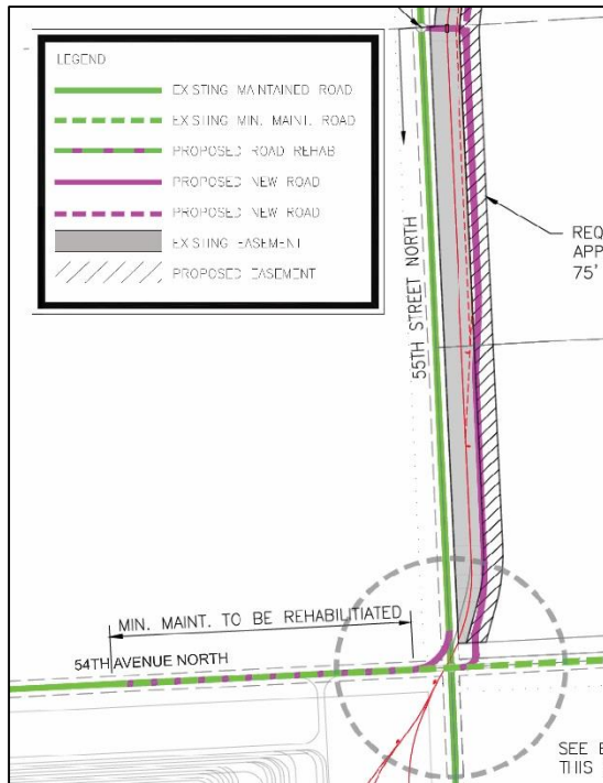
Figure 46: Proposed Rail Connection to NPN Site
