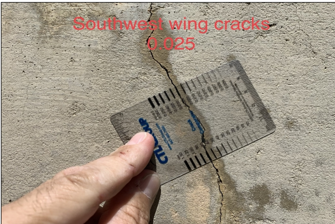
SW wing crack .025
