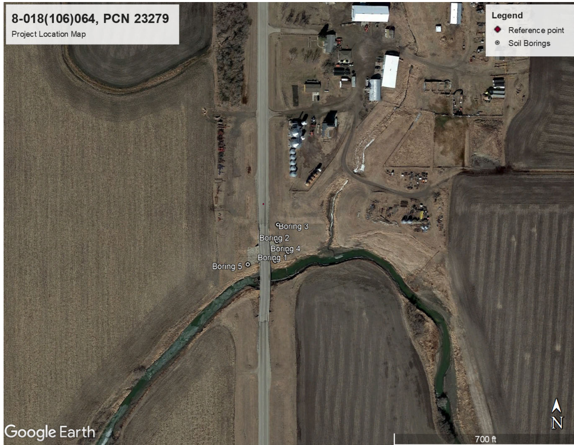
Figure 1 – Project Location and Soil Boring Locations
