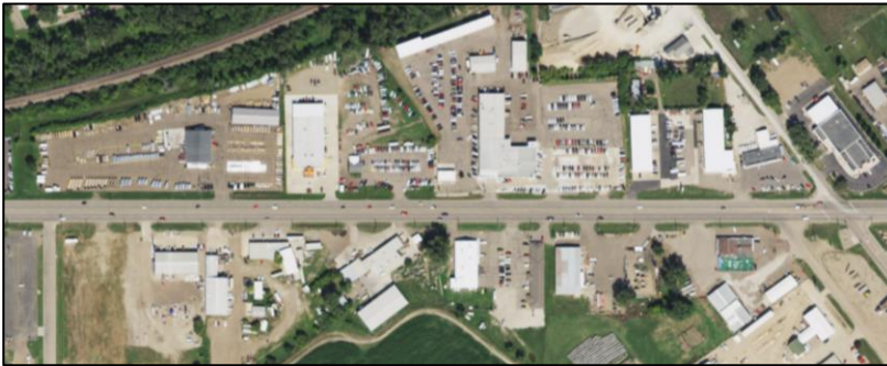
Strip Development (many lots with direct access to the arterial), DON'T DO THIS
