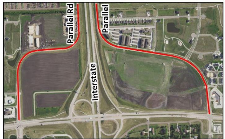
Parallel Roads Curve Farther From Interstate
